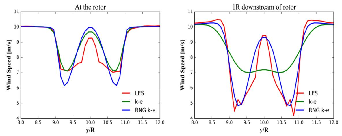
Figure 2. Stream wise velocity at hub height along the transversal direction produced by the polynomial method using two different closure models and state of the art LES simulation, at the rotor position and 1R downstream of the rotor position.
